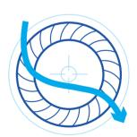
A Cross-flow turbine admission can have one or two compartments. The compartmentalization of **the inlet valve system ensures the turbine's efficiency when used under low flows.** JLA Cross-flow turbines are designed to operate over a wide range of flow rates while guaranteeing a minimum efficiency of 75% to 80%.
